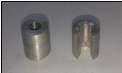
Figure. 3.5.4 Vortex tube Nozzle, Diaphragm Dia (inner, outer) = 7mm, 18mm,length =13mm
