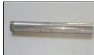
Figure. 2.3.3 Vortex tube Nozzle, Diaphragm Dia(inner, outer)=7mm,18mm,length=13mm
