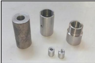
Fig: 3.5.1 Vortex tube cold and Hot chamber, Nozzle, Diaphragm, Adapter
