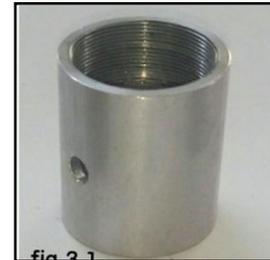
Figure. 3.5.3 Vortex tube Hot chamber Dia (inner, outer) =40mm,45mm
